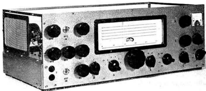
The complete receiver for 432 and 1296 Mc/s for which G3HBW received the Silver Plaque at the R.S.G.B. International Radio Communications Exhibition in 1962.
