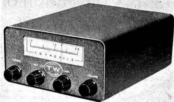
The Withers "Topmobile" transistor receiver for 1.8-2 Mc/s. The "Twomobile" is similar in appearance. Both receivers measure 6 in. wide, 6½ in. deep and 3 in. high.
